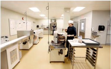
This new 3,800-square-foot renovation features sheet vinyl flooring, FRP walls, and stainless steel kitchen areas. Additionally, an upgraded HVAC system, with precise humidity control was installed to create a stable, more consistent environment for the chocolatiers.
